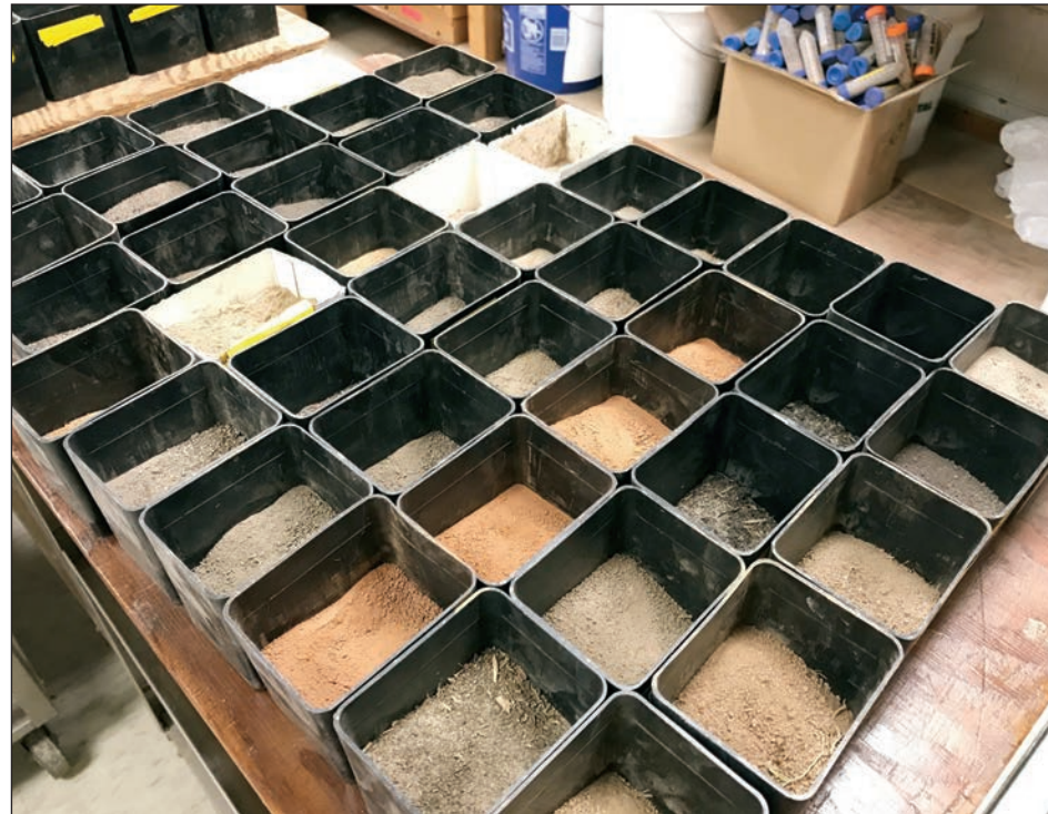
Soil samples that have been dried, ground and prepared for further testing at the LSU AgCenter Soil Testing and Plant Analysis Lab. Photo by Kyle Peveto/LSU AgCenter
